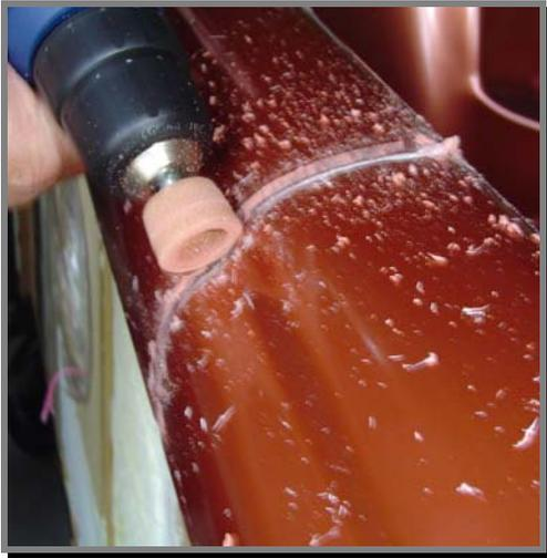
When starting this type of repair, you must first terminate the crack. This will prevent further cracking after the repair. Using a drill fitted with a cutting tool, remove all of the material and open up the ends. It is necessary to cut the sides at a 45° angle.
