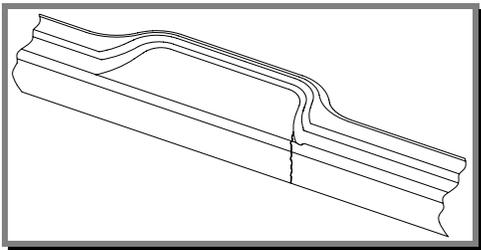
Cracks can occur on any part of the bartop. When this happens, the shell must be reinforced on the backside as well as the front side.
