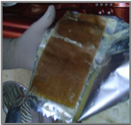
Using latex gloves, open the Zip Patch™ by carefully peeling away one side of the foil pouch to expose one surface of the patch. Spray the exposed patch surface lightly but completely (including the corners) with the activator. The patch will darken in color when it is properly activated.
