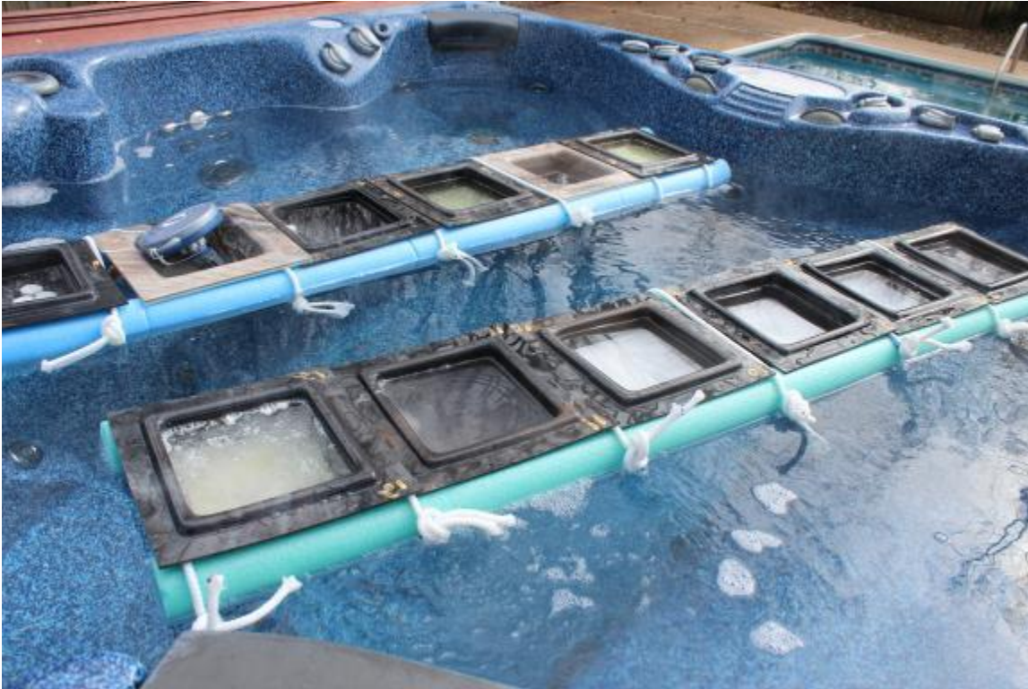
Mini spa testing utilizing a large spa as a water bath to maintain typical spa water temperatures Spa temperature was set at 103F
